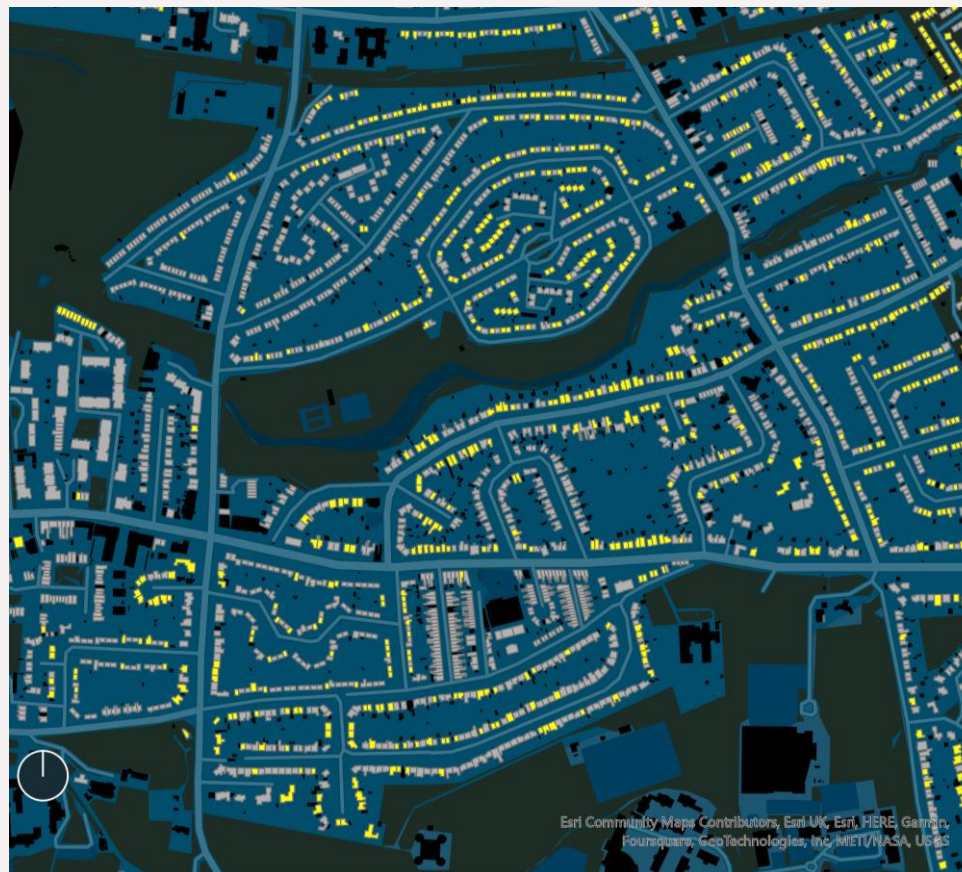
Dwellings with potential suitability for rooftop solar PV around Hull Road Park highlighted in yellow
